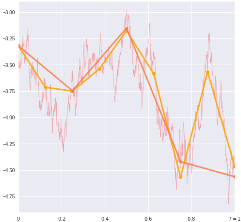
Figure 3.2: The plot shows the fine Euler-Maruyama approximation (bright orange) and the corresponding coarse one (orange) for the Multilevel data \mathfrak{Z}^3 = (X, \varphi(\mathcal{S}_8^{8, X}) - \varphi(\mathcal{S}_4^{4, X})) . The true trajectory of the solution to the stochastic differential equation is shown in red as a comparison.
